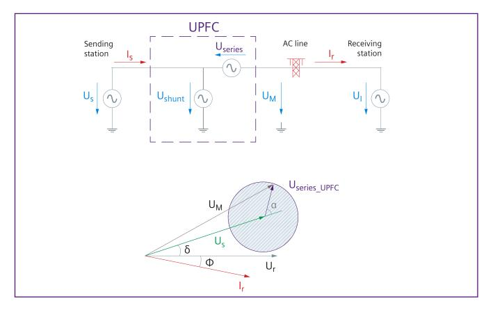
This is where UPFC outperforms other flow management components. In the field of dynamic load flow management, it supplies fast response in terms of active power management, coordinated reactive power control and can insert active damping to ensure stability.
