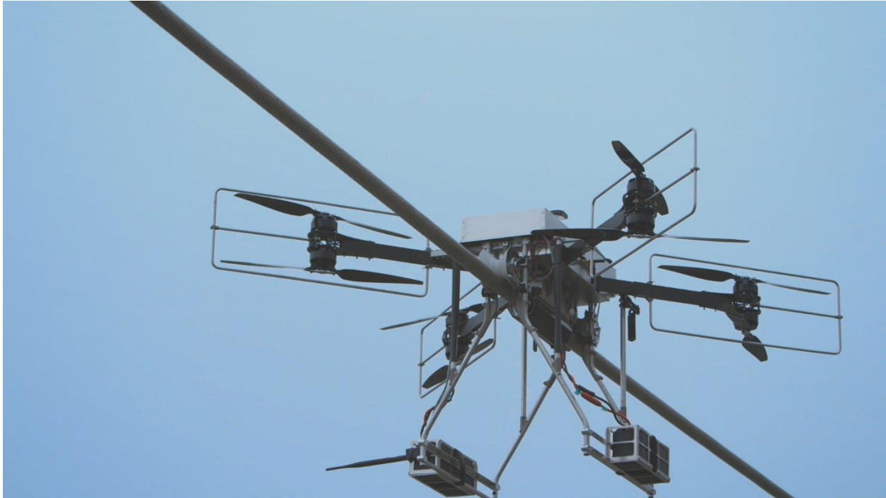
UAV equipped with LineCore sensor, by MIR Innovation, a subsidiary of Hydro-Québec, that is able to detect the first signs of conductor corrosion in a non-destructive way. Photo credit: Hydro-Québec
